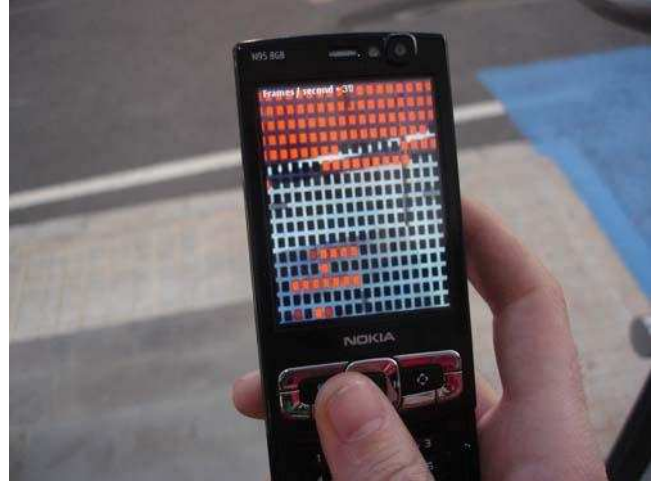
Fig. 1: An example of the binarization and grid sampling processing running on a Nokia N95 at 31 fps
