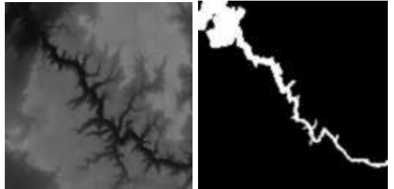
Figure 9. Left: Top view of second test mesh containing an applied texture with a river flow. The gray level indicates the elevation of each point. Right: Energy reduction mask to preserve the river area.
