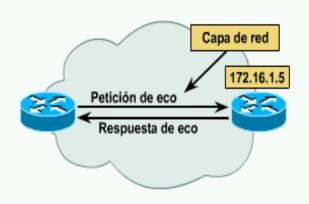
Router>ping 172.16.1.5 Type escape sequence to abort. Sending 5, 100 byte ICMP Echos to 172.16.1.5, timeout is 2 seconds: 11111 Success rate is 100 percent, round-trip min/avg/max = 1/3/4 ms Router>
