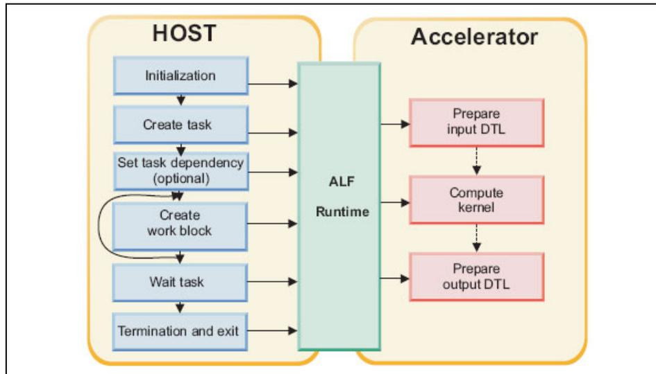
Figure 4-13 The host and accelerator sides
