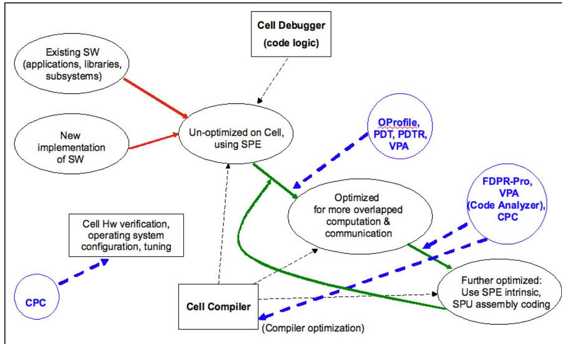
Figure 5-25 Typical Tools flow
