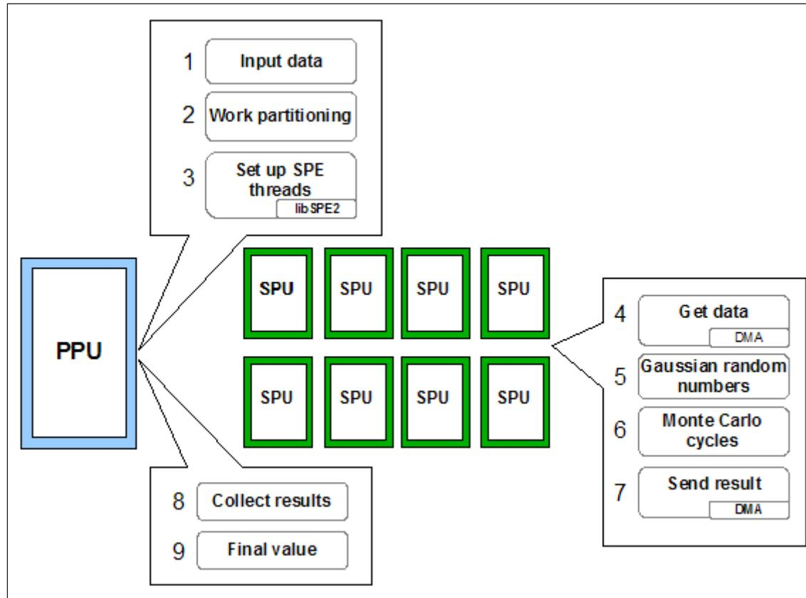
Figure 8-1 Logical steps: parallelizing the Monte Carlo simulation
