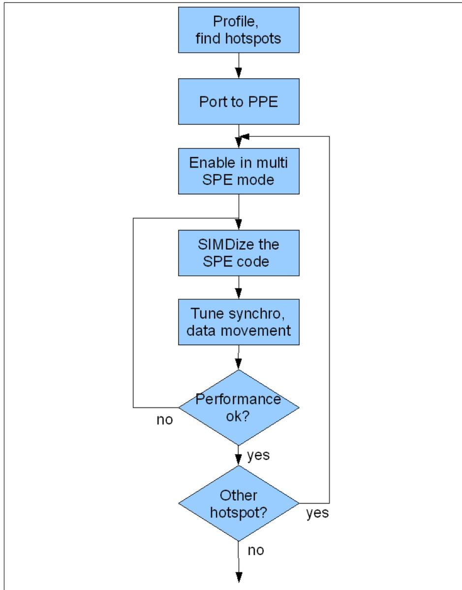
Figure 3-9 General flow for enabling an application on Cell BE
