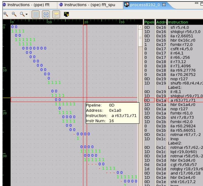
Figure 6-14 Cell Pipeline tab
