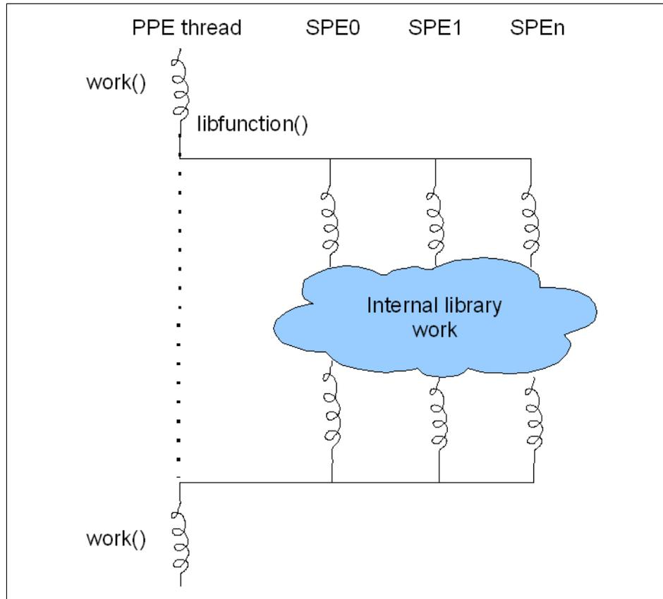
Figure 3-12 A typical work flow for Cell BE tuned workload libraries
