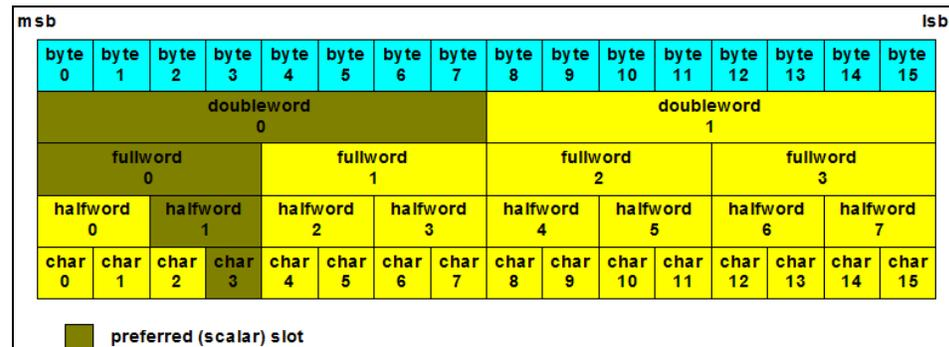
Figure 4-6 Scalar Overlay on SIMD in SPE
