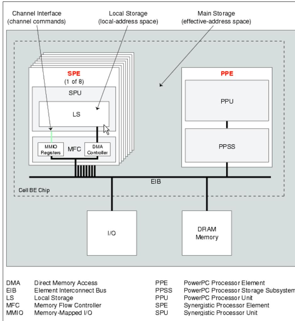
Figure 4-1 Cell BE storage domains and interfaces
