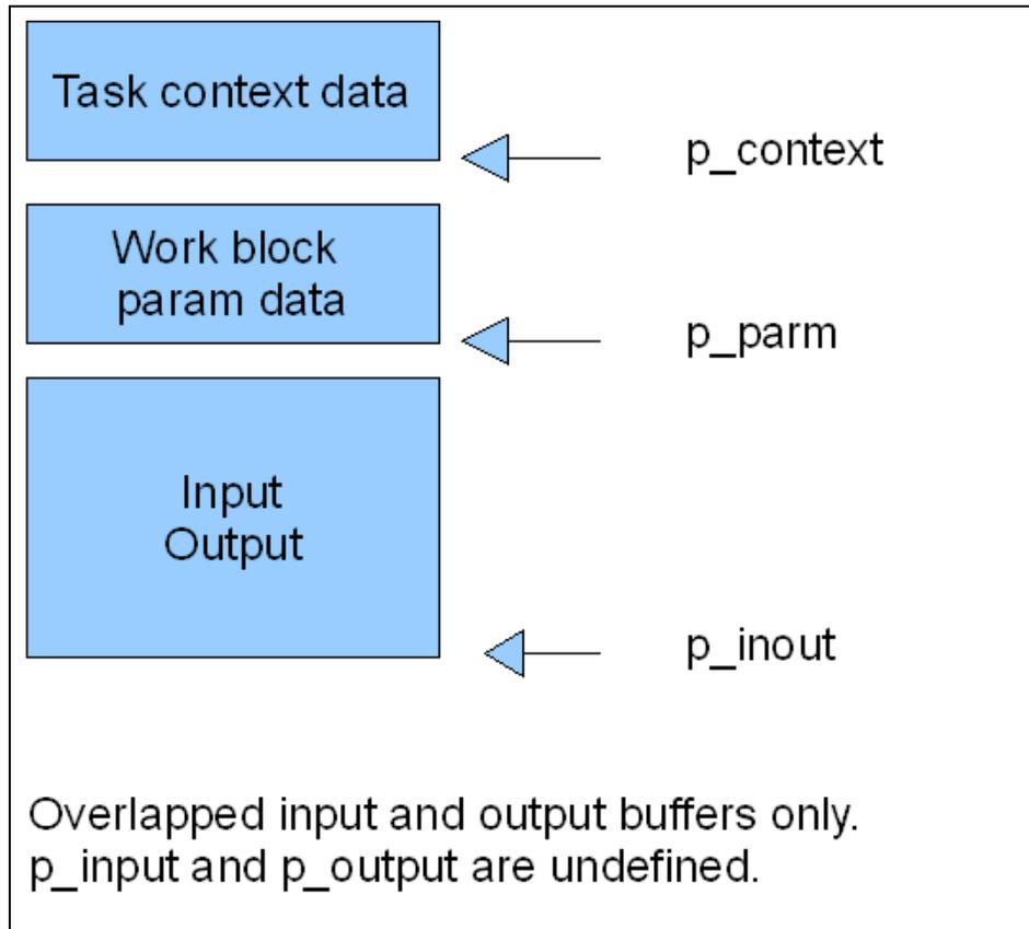
Figure 4-16 Memory map with a single input/output overlapped buffer
