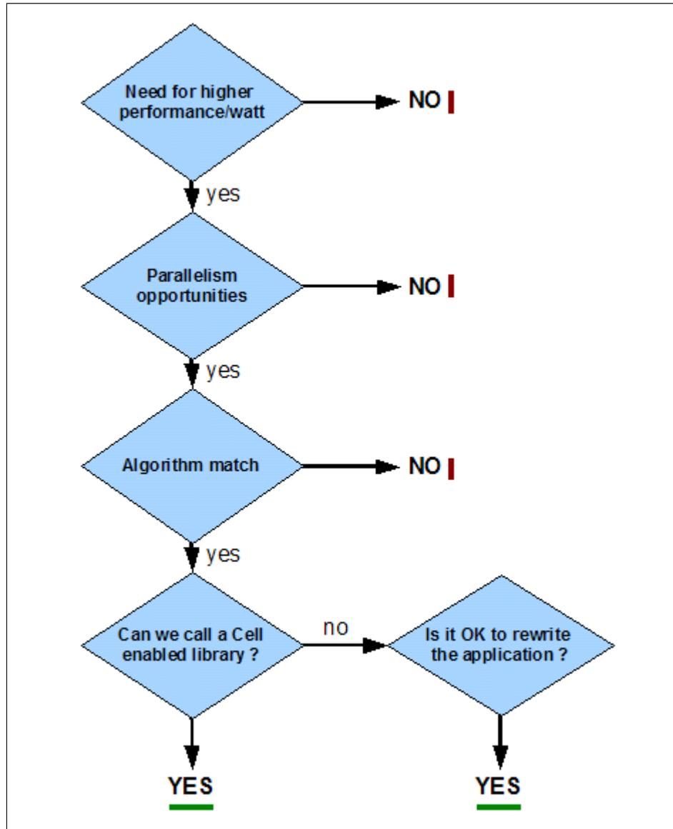
Figure 3-4 Is the Cell BE a good fit for this application
