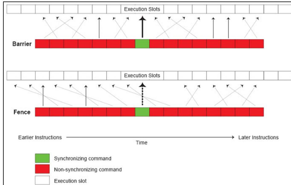
Figure 4-4 Barrier and fence effect
