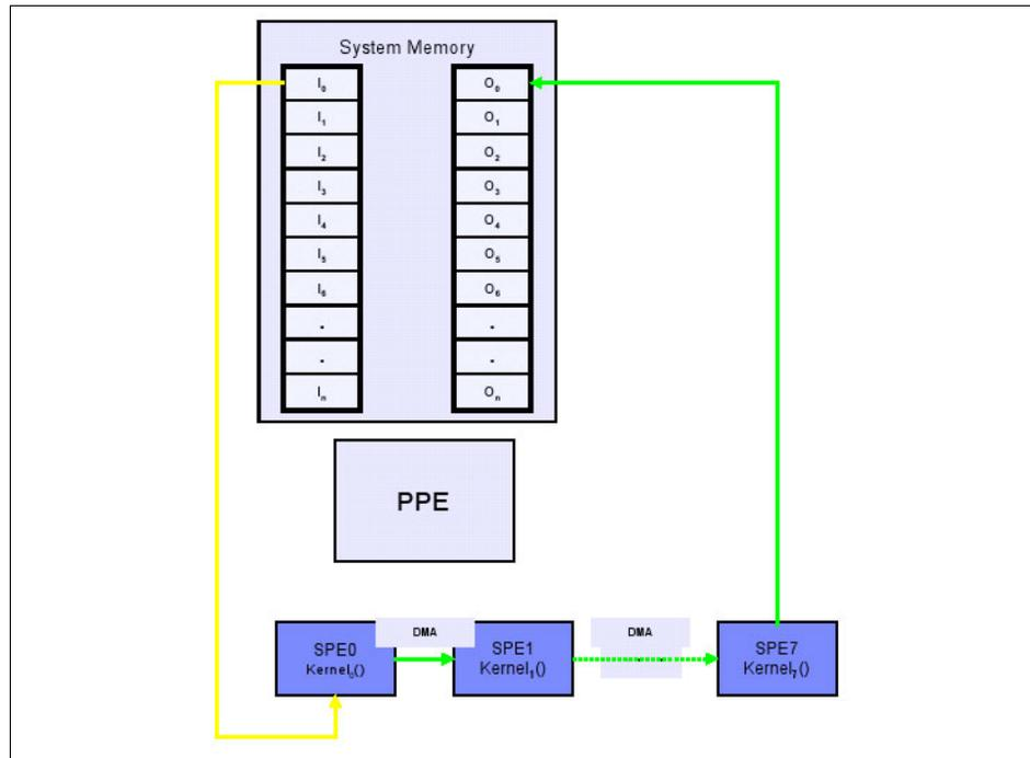
Figure 3-7 The pipeline model
