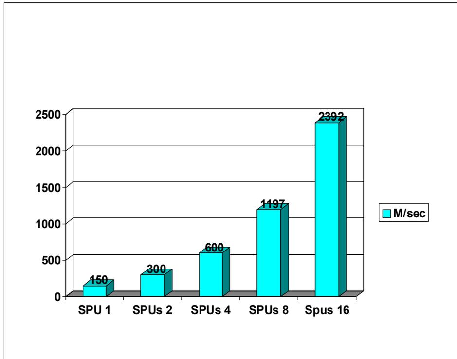
Figure 8-2 Performance of Monte Carlo simulation on QS21.
