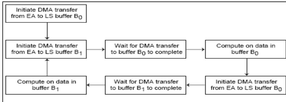
Figure 4-3 Double buffering scheme
