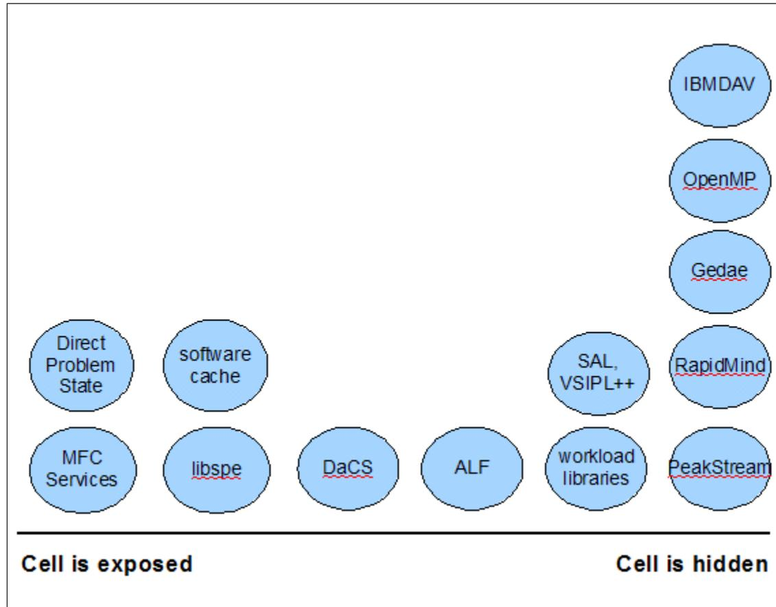
Figure 3-3 Relative positioning of the Cell programming frameworks
