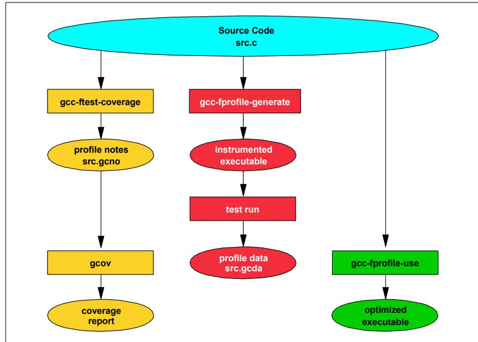
Figure 5-4 Profile Directed Optimization process
