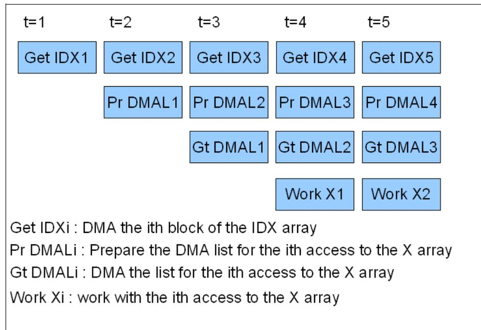
Figure 3-15 Software pipelining and multi-buffering
