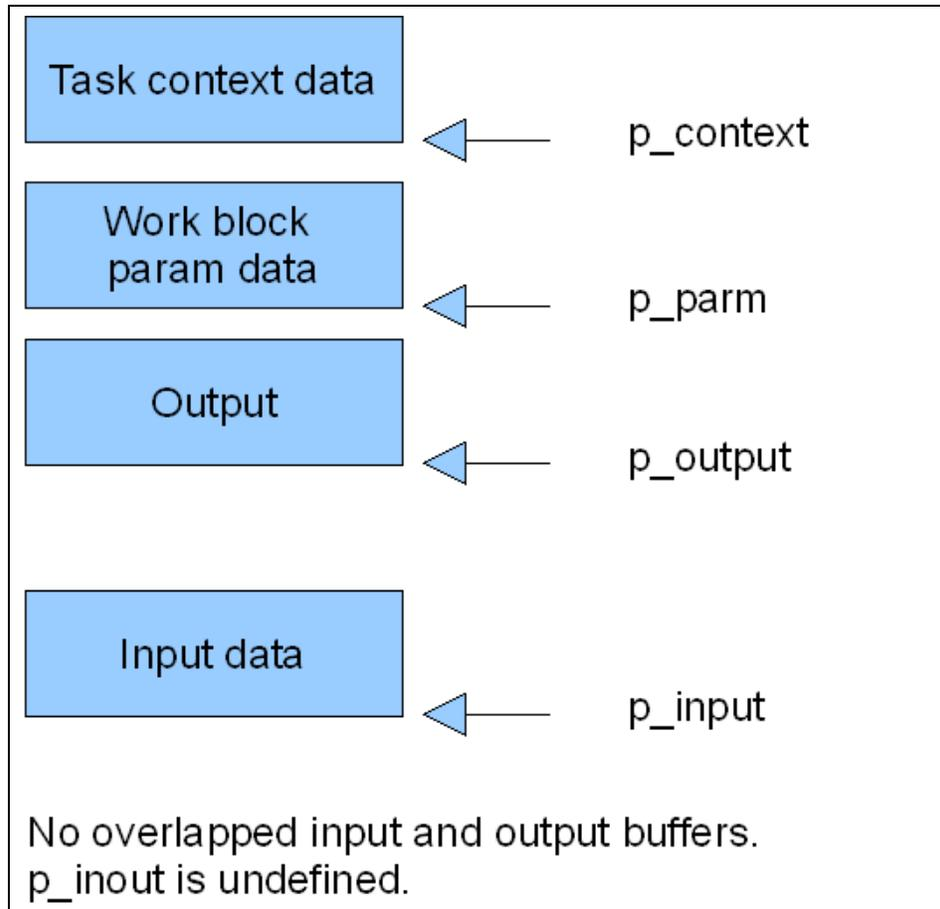
Figure 4-15 Memory map without overlapped input/output buffer
