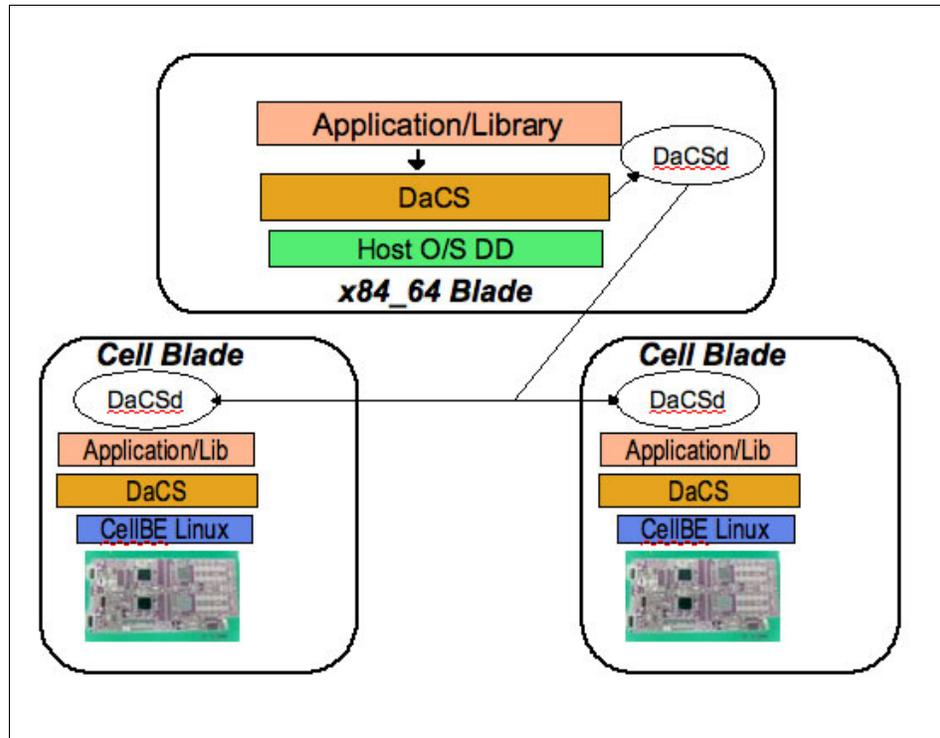
Figure 7-6 Hybrid DaCS architecture
