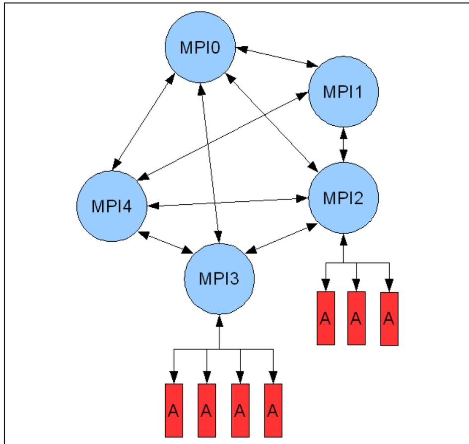
Figure 4-10 Possible arrangement for a MPI - DaCS application
