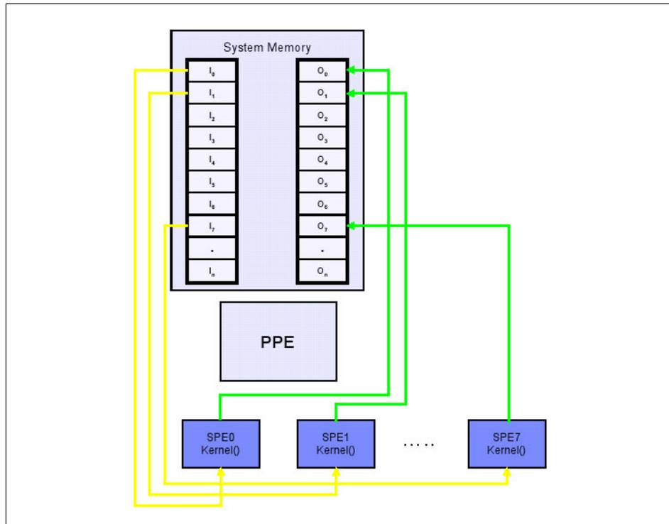
Figure 3-6 The streaming model
