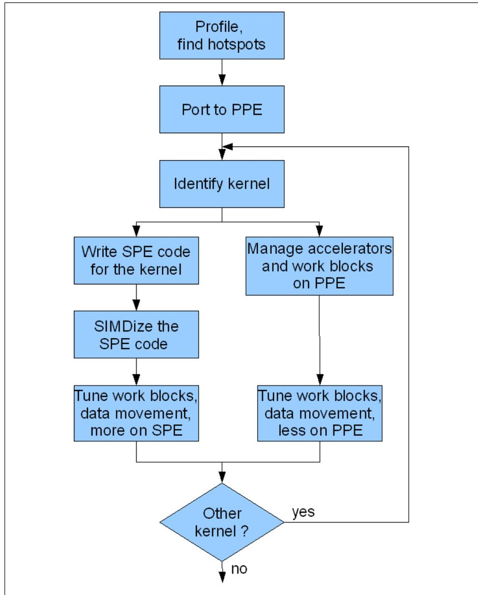
Figure 3-11 Enabling a Cell BE application with ALF
