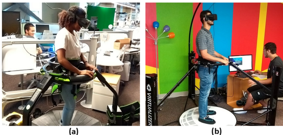
Fig. 5. Participants during the experimental session testing the BODT-Virtuix Omni (a) and FODT-Cyberith Virtualizer VR (b) platforms.
